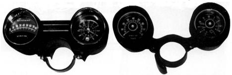
Just to complicate things a bit more, there were three different tachometers for each style. These were the 6000 max rpm - 6 cylinder, the 6000 max rpm - 8 cylinder, and the the 8000 max rpm - 8 cylinder High Performance. To determine whether a 6000 rpm tacho is a 6 or 8 cylinder version, remove the two screws from the rear of the housing, slide the tacho out and look for 6 cyl or 8 cyl stamped on the back.
