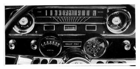
To determine which Rally-Pac is right for your early Mustang; if your car is a 19641/2 or a standard 1965 car with the above style instrument panel, then you need the hooded Rally-Pac. If your Mustang uses the five-gauge instrument panel as per below (which is standard on the 1966 car and comes with the GT Equipment Group and/or the Décor Interior on 1965 cars), then it's the low-profile version that you will be looking for.
